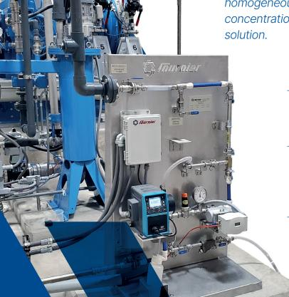
Capable of effectively activating and fully blending a homogeneous polymer solution with a 0.1% to 0.45% concentration, starting from a 40% to 55% neat polymer solution.
